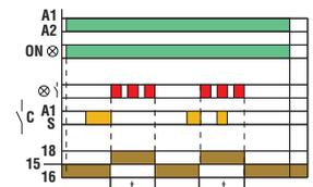
Flasher, starting with OFF (pause) interval. Equal timing recycle
